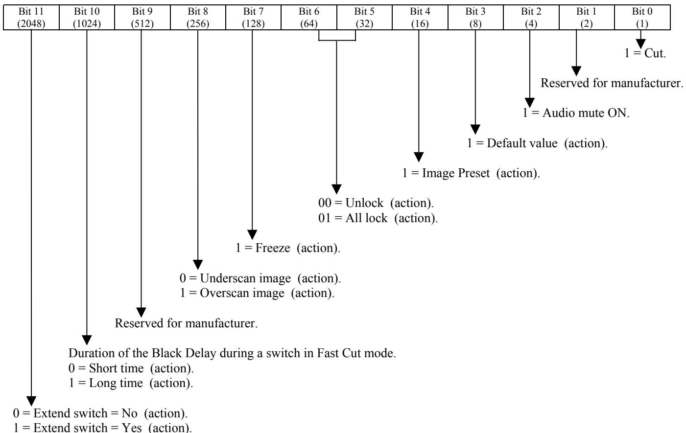
**NOTE:** To modify an adjustment you should first read the value of the command, then modify the value of the corresponding bit without modifying the value of the other bits, and then return the new value.
