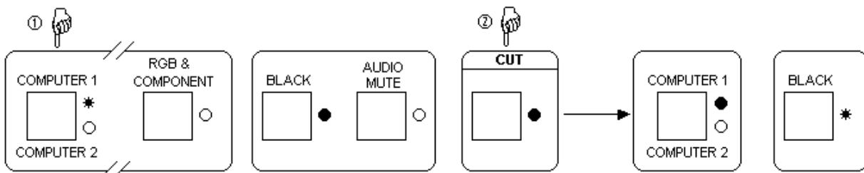
③ Pre-select a video input (C.VIDEO 1, C.VIDEO 2, S.VIDEO 1, S.VIDEO 2, or RGB & COMPONENT) with the front panel selection keys (the corresponding LED is blinking).
